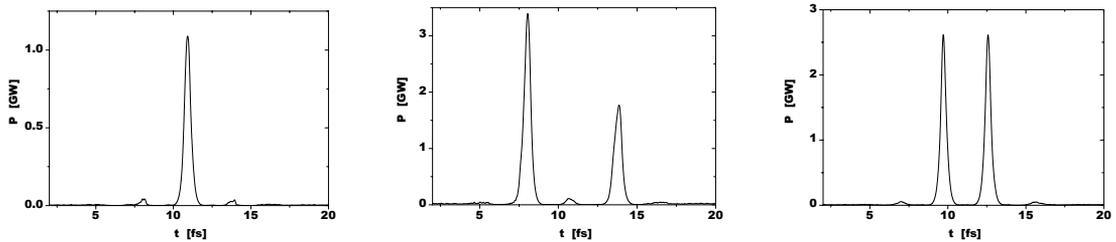
Figure 5: Averaged temporal structure of the radiation pulse behind monochromator tuned to single spike (left plot) and two pulse sequence selection (middle and right plots).
