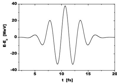
Figure 2: Energy modulation of electron bunch at the exit of the modulator.
