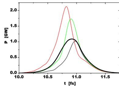
Figure 6: Temporal structure of the radiation pulse behind monochromator tuned to single spike selection (mark  $M_1$  in Fig. 4). Thin curves are single shots, and bold curve is average over many pulses.
