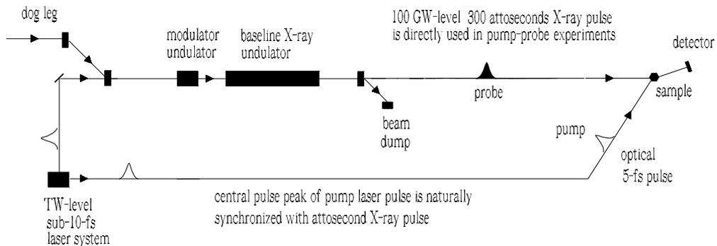
Figure 7: Scheme for femtosecond resolution pump-probe experiments based on the generation of the 100 GW-level attosecond X-ray pulses directly from X-ray SASE FEL.
