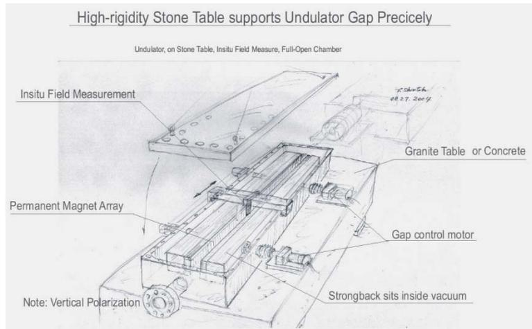
Fig. 4. Granite table as the support structure of the undulator magnet. Massive granite will provide high rigidity against various deformation forces. In-situ field measurement will be performed by movable probe, whose linear guide has to be integrated into the chamber.
