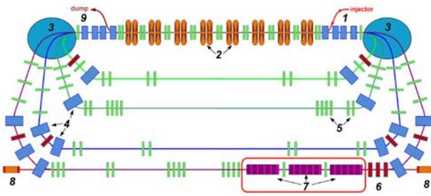
Figure 3: Scheme of NovoFEL installed on a four-track ERL: 1- electron injector, 2 - NRF cavities, 3 – round dipole magnet, 4 - rectangular magnets, 5 – quadrupole lenses with dipole correctors, 6 - quadrupole lenses, 7 - undulators of the electron outcoupling system, 8 - mirrors of the optical cavity, 9 - electron dump.
