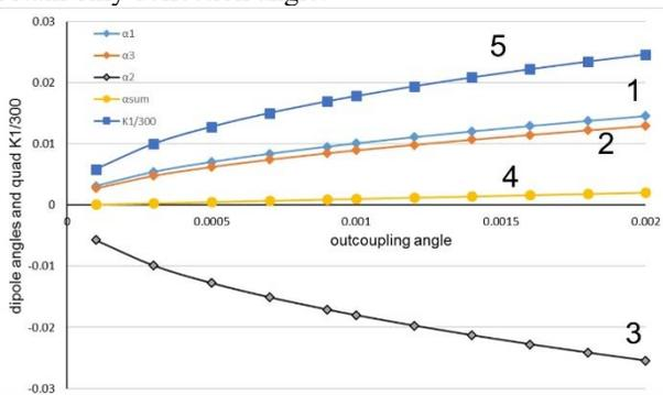
Figure 7: Achromatic bends parameters for the different outcoupling angles: 1,2 – dipole corrector’s angles, 3 – angle of the shifted quadrupole, 4 – total angle, 5 –  $K_1$  parameter of the quadrupole.
