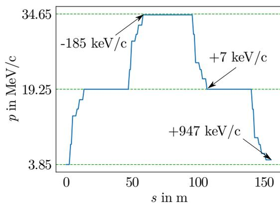
Figure 3: The acceleration/deceleration process is visualized for the case of a beam tracking with optimization on the first main linac transit, operating on-crest. The used energy gradients are identical to the ones used at the first test phase of the twofold ERL mode. Due to phase slippage, the acceleration/deceleration is not optimal for the subsequent main linac transits. The mentioned values are the deviations from the target momenta.
