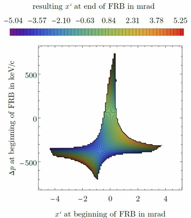
Figure 2: Two cross sections of the acceptance phase space of the first recirculation beamline (FRB). The variables are deviations at the beginning of the FRB, the values of the contour plot represent the resulting divergence  $x'$  at the end of the FRB.
