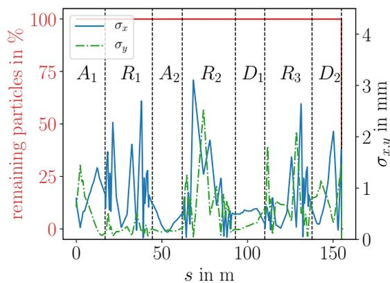
Figure 4: Beam losses and envelopes in the case of a beam tuning with optimization on the first main linac transit, operating on-crest. Highlighted sections: (A)cceleration, (R)ecirculation, (D)eceleration. Due to imperfect deceleration, the electrons can not be guided into the intended beam dump, but are lost during the last deflection due to beam rigidity.
