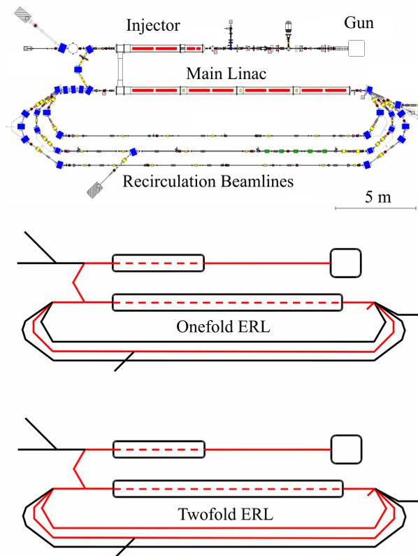
Figure 1: Floor plan of the S-DALINAC and schemes for the onefold and twofold ERL mode.
