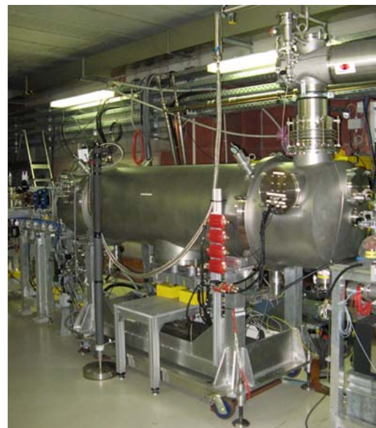
Figure 2: First of the two cryogenic modules at ELBE.
