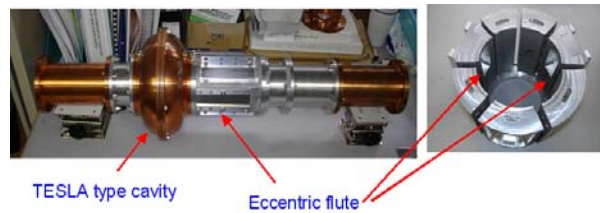
Figure 10: (Left) Picture of the test model of the EFB. (Right) Angularly divided EFB
