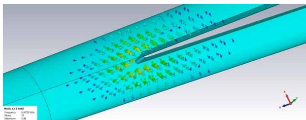
Figure 7: Unavoidable trapped mode. Electric force lines.
