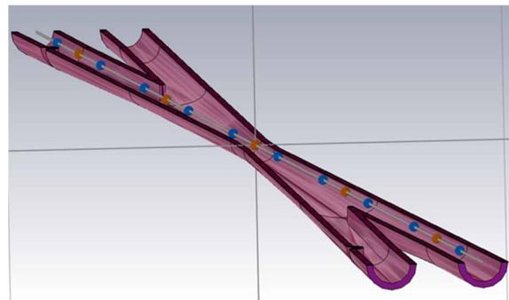
Figure 3: CAD model for the wake field calculations.
