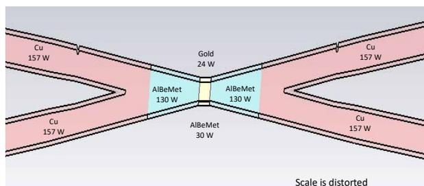
Figure 10: Heat load distribution in the FCC IR.
