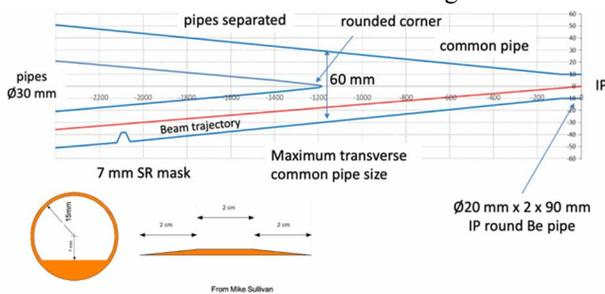
Figure 2: Last FCC IR geometry and SR mask shape.
