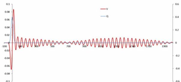
Figure 5: Wake potential of a 12-mm bunch passing the 10-m long beam pipe of the FCC IR.
