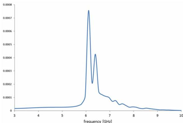
Figure 6: Spectrum of the wake potential
