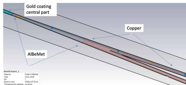
Figure 9: CAD model with different materials.
