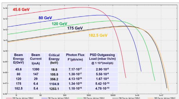
Figure 1: SR spectra: Units: Vertical: ph/s/m/(0.1% Bandwidth); Horizontal: eV; Intervals: Vertical: [106; 2·1014]; Horizontal : [4; 5·106]; Inset table: linear photon flux, and linear PSD rate at each energy.
