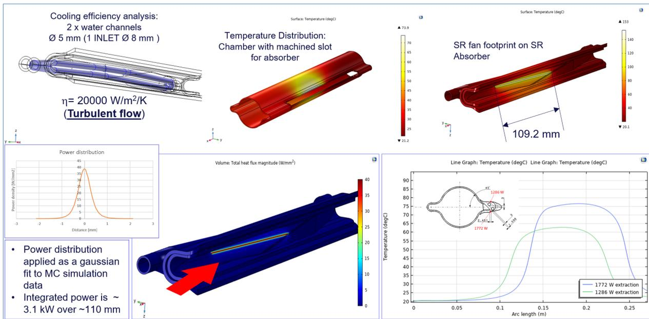
Figure 2: Composite figure showing results of calculations carried out for the SR absorbers; clockwise, from upper left: optimisation of turbulence vs pressure drop; temperature distribution near one SR absorber; temperature distribution along one absorber; wall temperature at the cooling channels vs length; SR power density along one absorber; vertical distribution of SR fan (from ray-tracing monte-carlo simulation, SYNRAD+ code).
