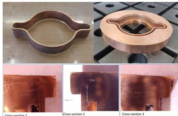
Figure 3: Short chamber extrusion, oval flange, and cross-section of the FSW tests, showing correct joining of the two parts.
