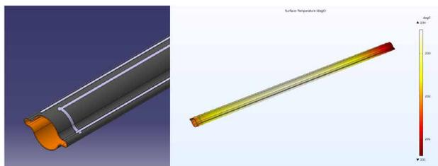
Figure 4: Left: CAD view of the chamber extrusion covered with insulating ceramic layer and sprayed Ti tracks; Right: Temperature distribution computed for a 5m-long chamber.
