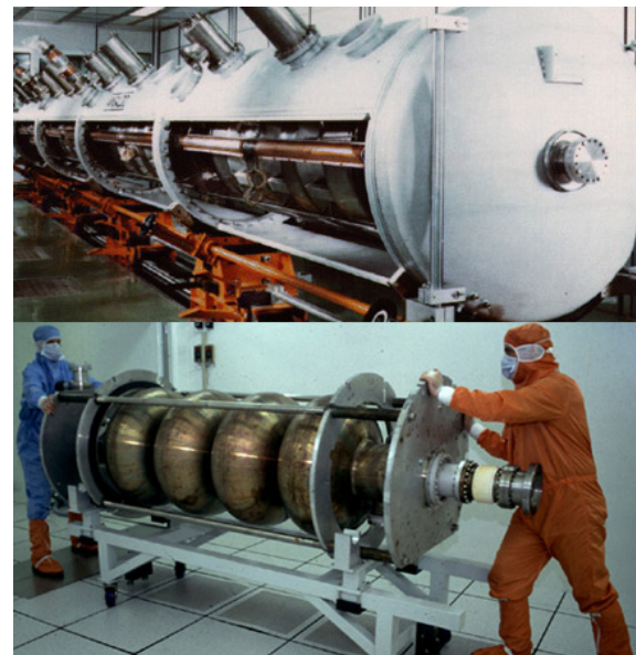
Figure 2: LEP2 cavities in industries during cryostating in large clean rooms of class 100/10.000.
