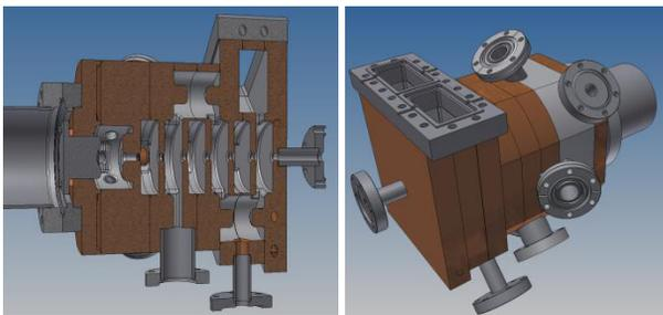
Figure 7: mechanical design.
