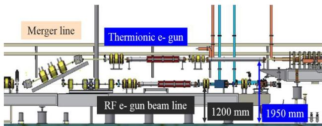
Figure 11: Thermionic gun and RF gun beam line.
