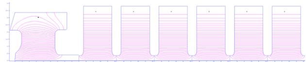
Figure 2: Designed RF gun cavities (SUPERFISH calculation result).
