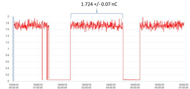
Figure 12: Beam charge stability of RF gun.
