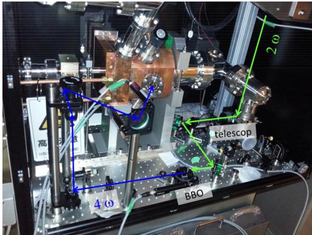
Figure 10: Laser injection component near the RF gun.
