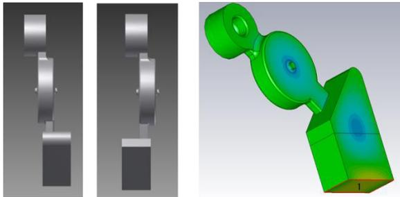
Figure 5: Two type couplers and calculation result.
