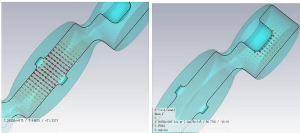
(a) Accelerating mode (b) Coupling mode
