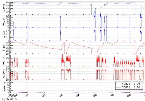
Figure 13: RF gun beam injection history graph.
