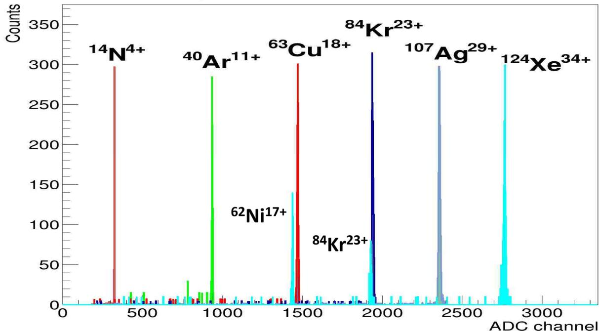
Using detectors, identified high charge state Ag and Xe from our ECR2 ion source.
