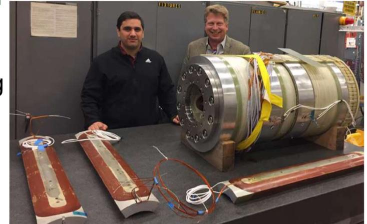
Quenches of sextupole magnet with new coil #9. Required current 450A.
