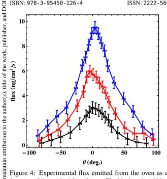
Figure 4: Experimental flux emitted from the oven as a function of the angle  $\theta$  for calcium. The black, red and blue plots are respectively measured at the temperatures 850, 875, 900°K.
