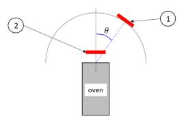
Figure 3: Sketch showing the positions of the quartz balance during the experiments. (1) The quartz describes a circle of radius 60 mm around the oven exit. The quartz and the oven axis form an angle with  $-\pi/2 \le \theta \le \pi/2$ . (2) The quartz is set 10 mm away from of the oven hole.
