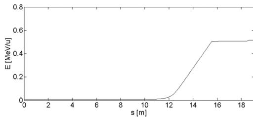
Figure 8: The energy of the oxygen beam along the SCL demo.
