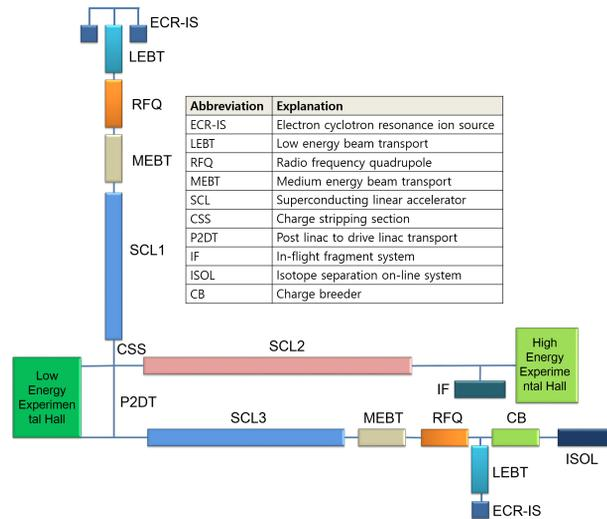
Figure 1: Schematic view of the RAON accelerator.
