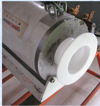
Central insulator, e = 3\text{mm} (2 parts) 60 kV: OK
