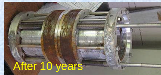
Remember: central core of the Booster (HT) To be inserted into the insulator
