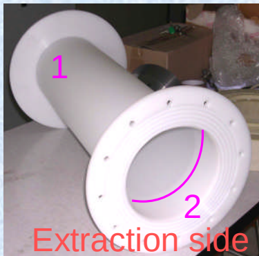
Central insulator, e = 3\text{mm} (2 parts) 60 kV: OK
