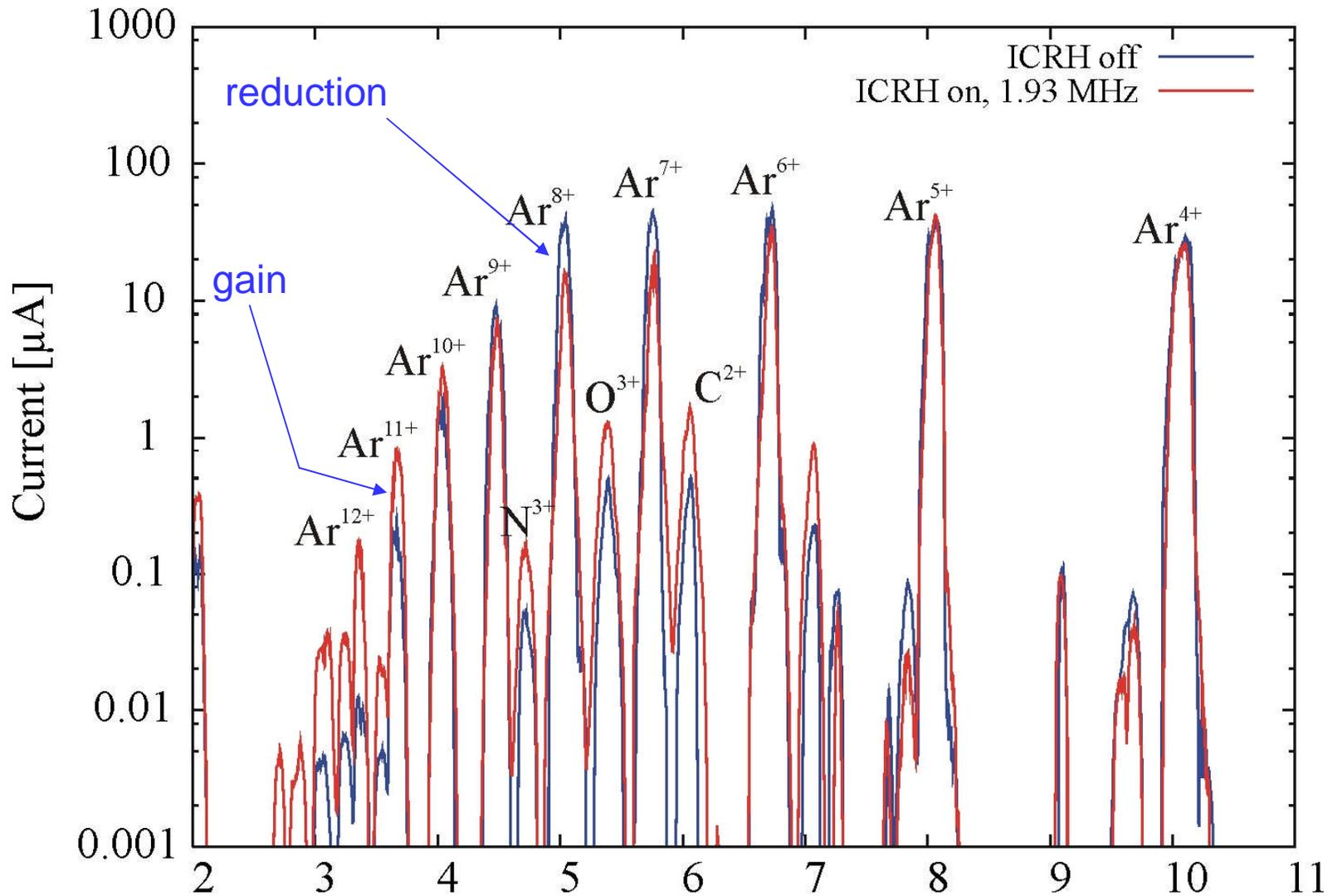
Outgazing from the volume between the Cu-electrodes and the  $\text{Al}_2\text{O}_3$ -cylinders causes important fluctuations of all currents measured !!
