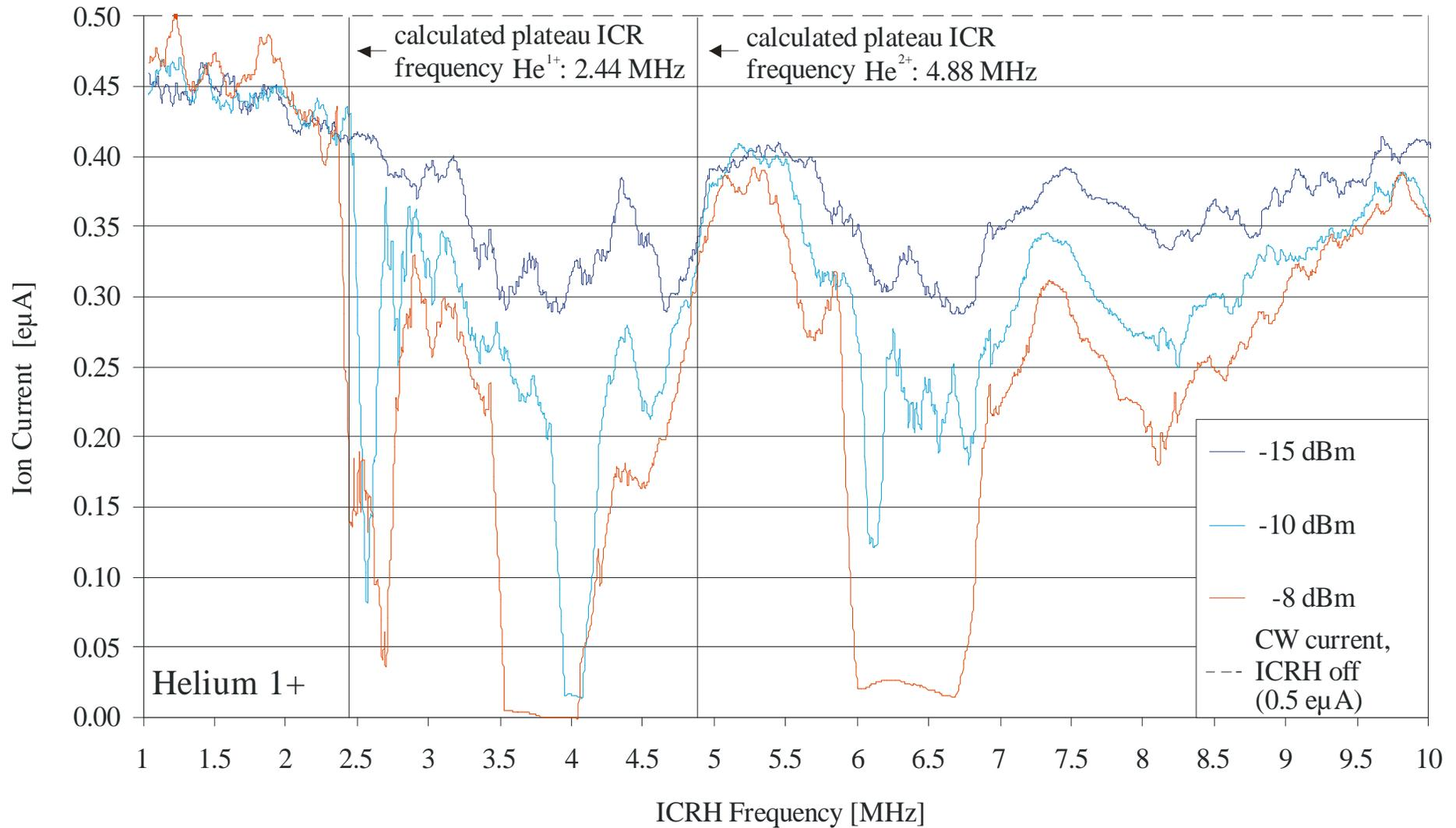
RF is varied in steps of 100 kHz from 1 to 10 MHz at B = 0.64 T
