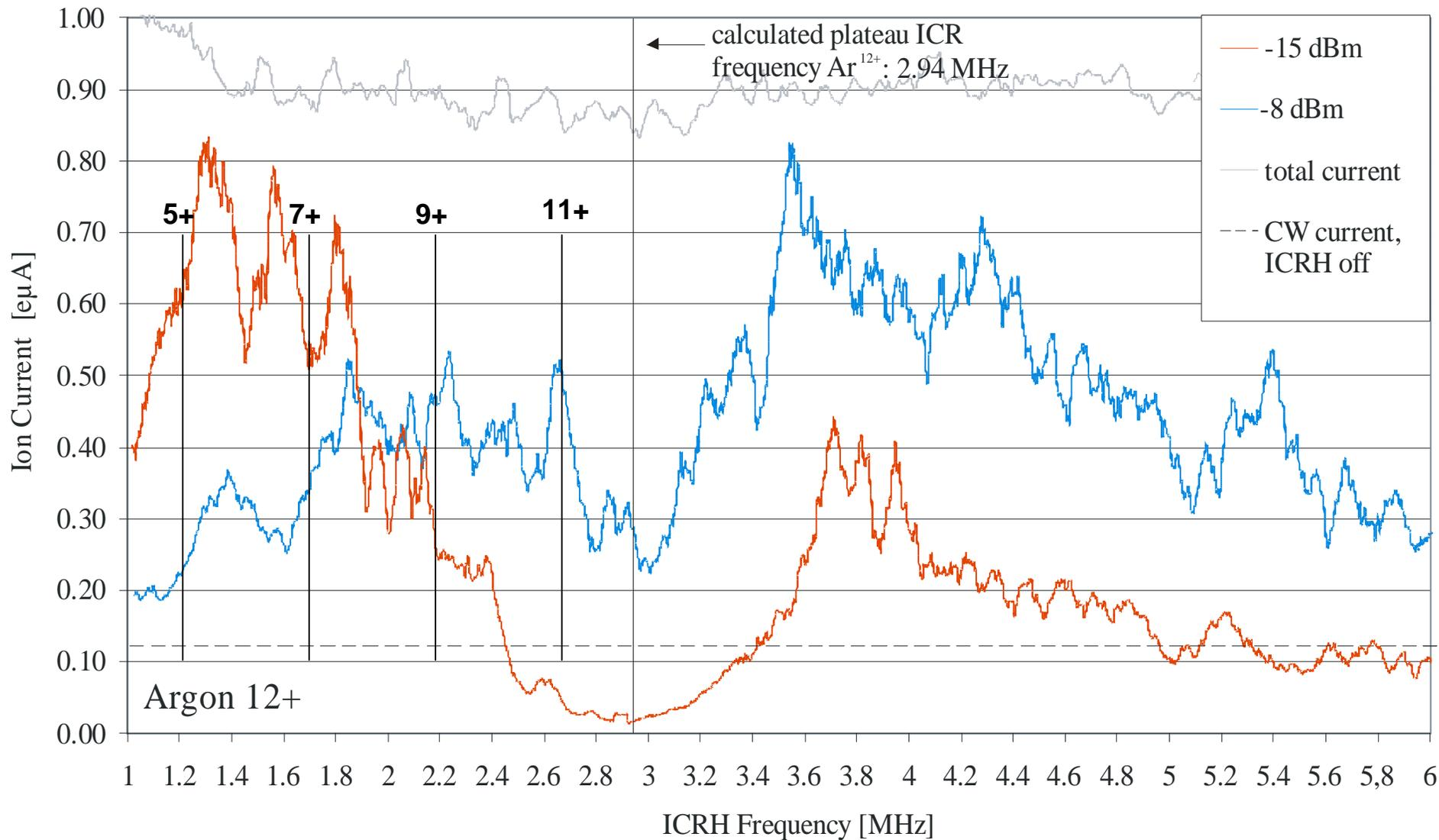
ICRH-frequency is stepped by increments of 100 kHz
