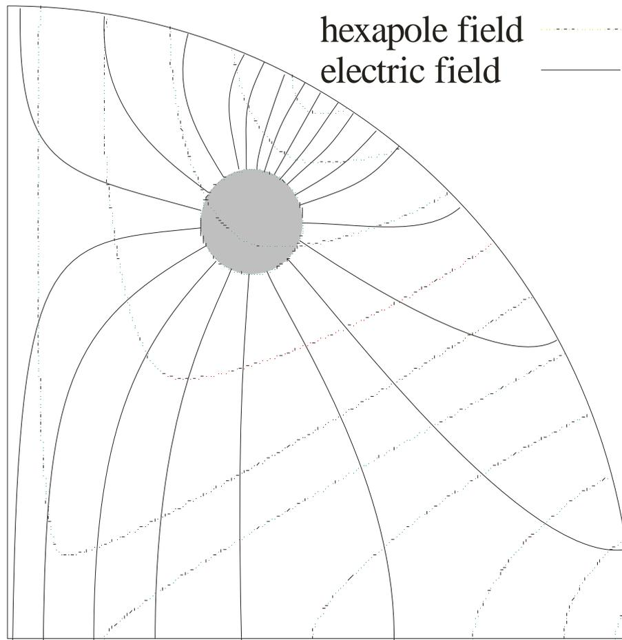
The electric field can penetrate where the electric field  $\perp$  hexapole field
