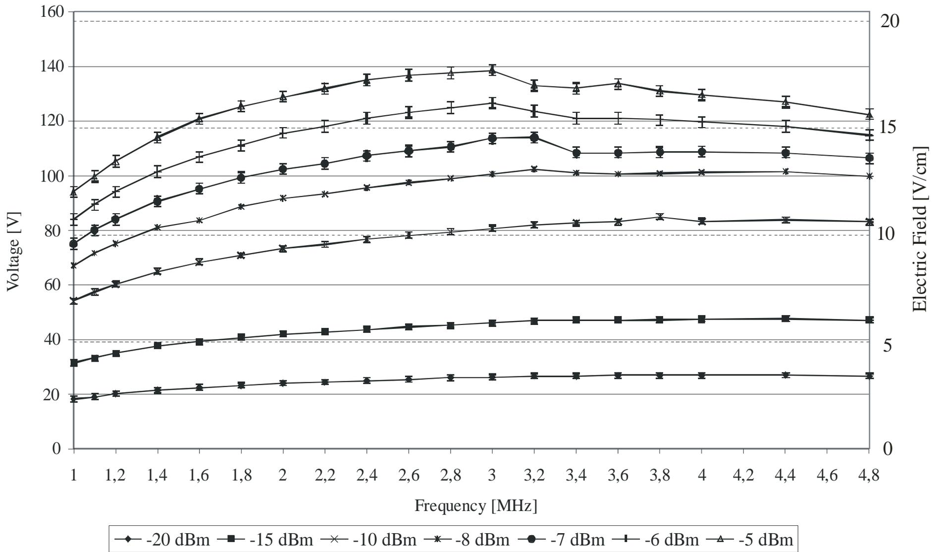
**Nearly flat RF-field amplitudes as function of frequency and damping**
