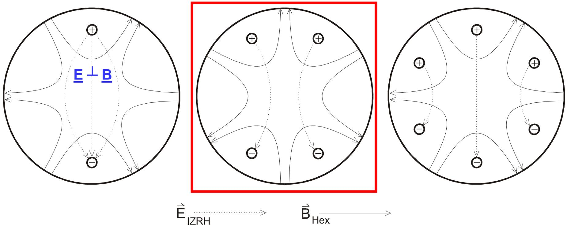
Our choice with smallest electric field between electrodes and wall
