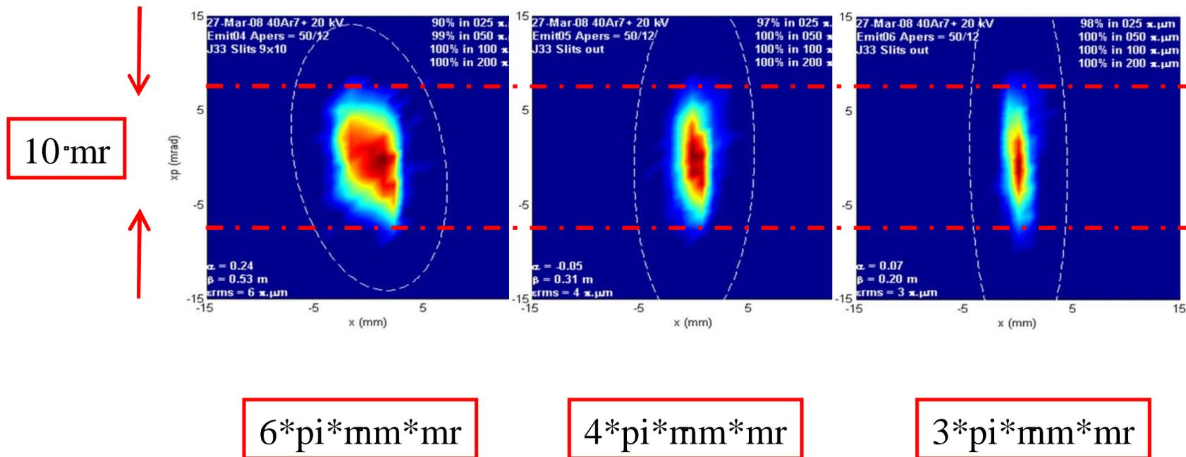
When divergences  $< \sim 10$  mr, as they are for many of these measurements, the calculated emittance values depend only on the beam width.
