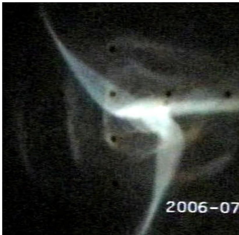
“Rings” morph into “Stars” by varying the focusing strength of lenses.
