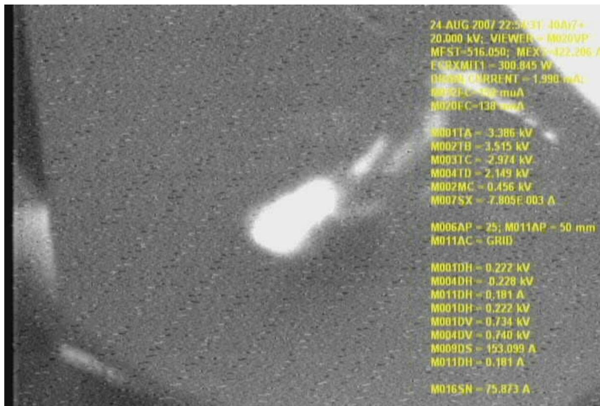
The External Sextupole “brings in” highly aberrated beam, but doesn’t affect the “core” at all(!)
