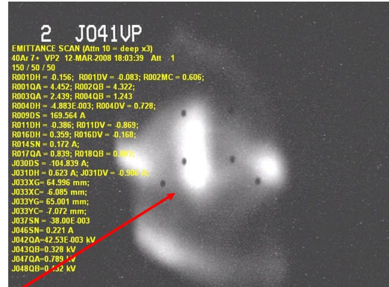
This central piece of beam is not being significantly cut by apertures. There seem to be 3 similar low-emittance pieces, but on different trajectories. The apertures cut 2 of the 3 (plus a “cloud”) away.
