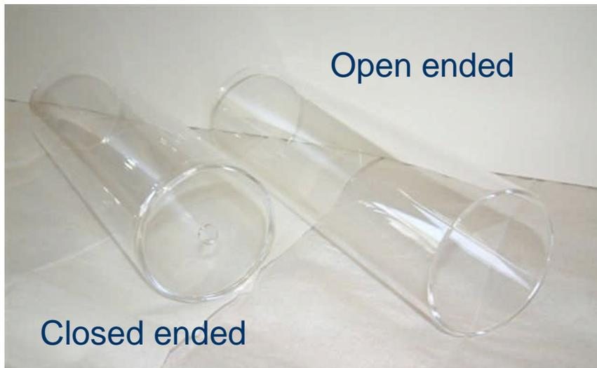
Closed Liner: 10mm opening on axis to allow for beam extraction and the other end a 5mm hole to allow for the introduction of a sample gas.
