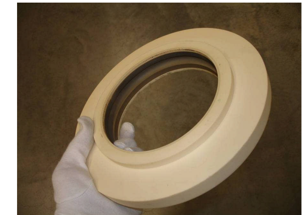
Figure 6: Isolator after 3 weeks of CO_2 operation of the first extraction system that HIT bought with the source (e.g. Figure 5)
