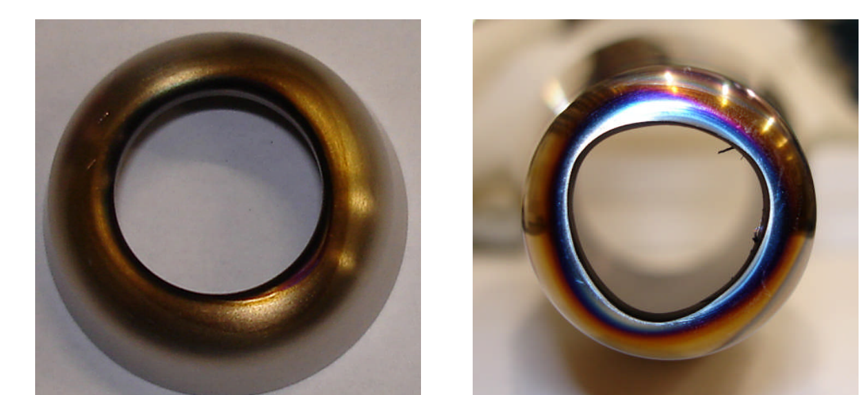
Figure 9: Left the new design of the titanium bias cap after 6 months of operation (still o.k.), right the old design made of molybdenum after 3 months of operation (broken).
