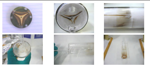
Figure 2: The top images show residual surface contamination on the plasma electrode and on the plasma bottle. The lower images show the ion source bottle after atmospheric baking at 1000°C for 2 hours. Note that the plasma electrode, and the rear of the plasma bottle both display a clean region which is in line with the loss zone of the plasma and is surrounded by the contaminants.
