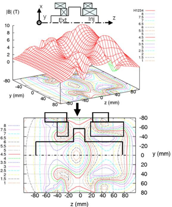
Figure 4: 3D simulation. Magnetic field  $|B|$  in the Oy-Oz plane.
