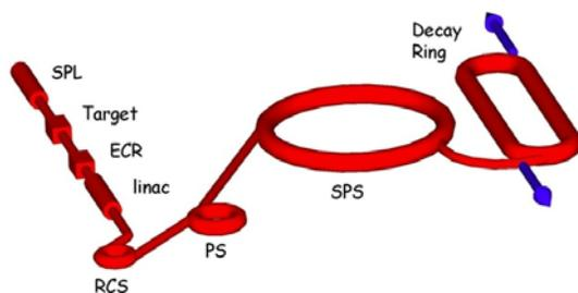
Figure 1: Baseline scenario of the beta-beam accelerator.
