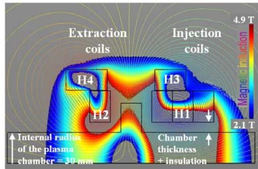
Figure 3: 2D simulation with pitch change configuration of H1. Half of the plasma chamber is represented.
