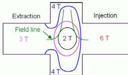
Figure 2: Magnetic field expected in the plasma chamber.
