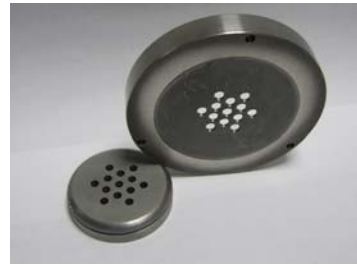
Fig. 4. 13-aperture extractor (photo). a) General view; the holes in plasma electrode can be seen at foreground. b) Electrodes of the extractor.
