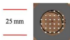
Figure 3: The Artemis-B grid is placed behind a 25 mm diameter aperture. The grid holes are about 1.5 mm in diameter, and 4 mm between centers.
