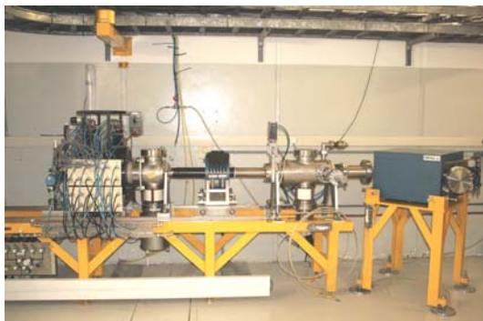
Figure 3: The Hahn-Meitner-Institute ECRIS4 source and the new beam-line, consisting of a solenoid, a diagnostic chamber and 90°-degree bending magnet.
