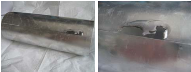
Figure 4: The ultra pure aluminum liner after losing thermal contact from the plasma chamber wall.
