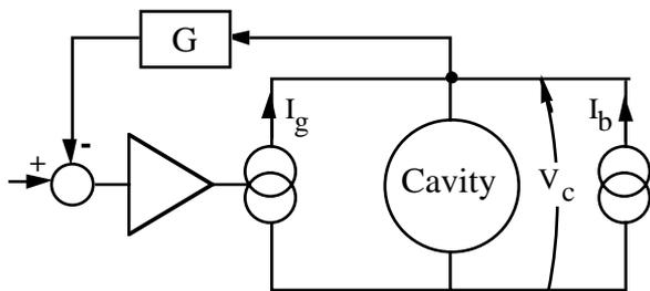
Fig. 2 : Schematic of the direct RF feedback
