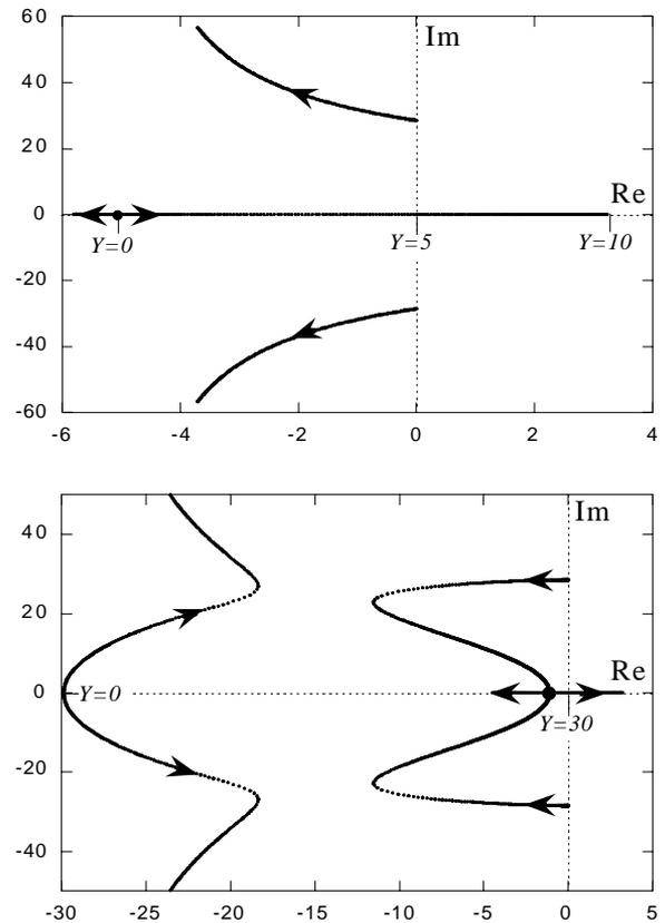
Fig. 3 : Root locus (variable is  $Y$ ), without (top) and with (bottom) RF feedback ( $G=5$ ).
