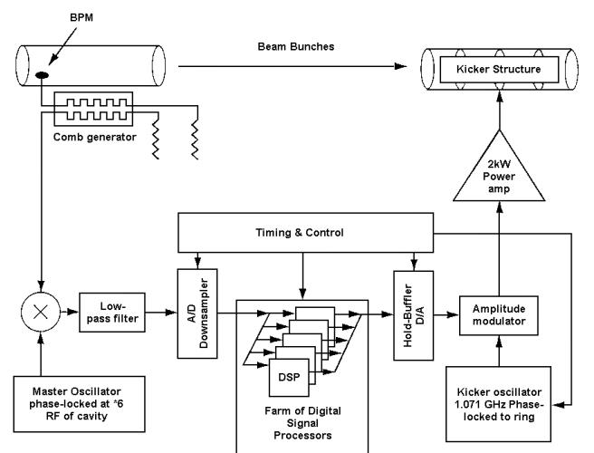
Figure 3. A block diagram of the Longitudinal Feedback System.
