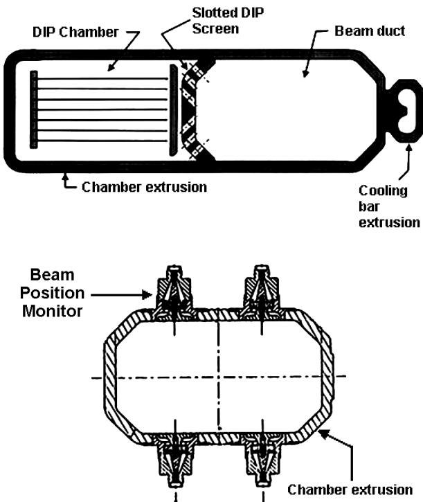
Figure 4. HER Arc dipole (upper) and quadrupole vacuum chamber profile.
