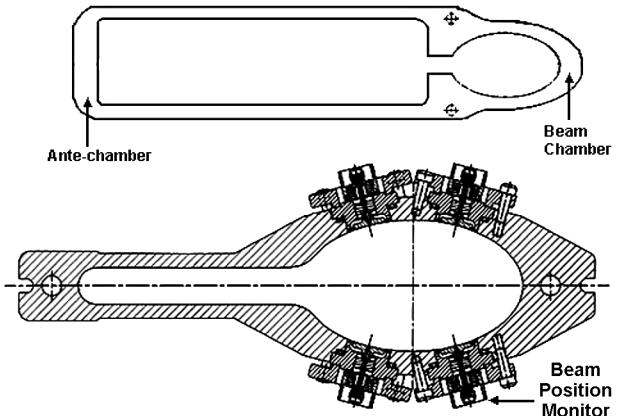
Figure 5. The LER Arc Magnet Chamber (lower) and pumping chamber. The Magnet Chamber is captured by the dipole and quadrupole. The Pumping Chamber, which houses the photon absorber, is downstream of each Magnet Chamber.
