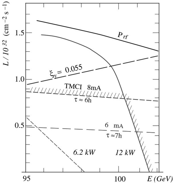
Fig. 3: Limits in the luminosity-energy plane for  $J_x = 1.0$ ,  $k_b = 4$  and  $102^\circ/90^\circ$  optics. Parameters:  $\epsilon_{x0} = 44.4$  nm at 100 GeV and  $J_x = 1.0$ ,  $\kappa = 1$  %,  $\beta_x^* = 2$  m,  $\beta_y^* = 0.05$  m. Lowest hard limits are shaded.
