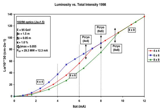
Fig. 2: Expected luminosity as a function of the total current  $2I_0$  for  $k_b = 4, 6, 8$ . The beam-beam limit  $\xi_y = 0.055$  is reached on the oblique straight line. The 1998 cryogenics limit is indicated. The rf power limit is reached at 12 mA.
