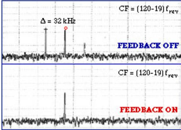
Figure 6: Beam spectrum without and with feedback in the positron ring, 30 bunches, 70 mA
