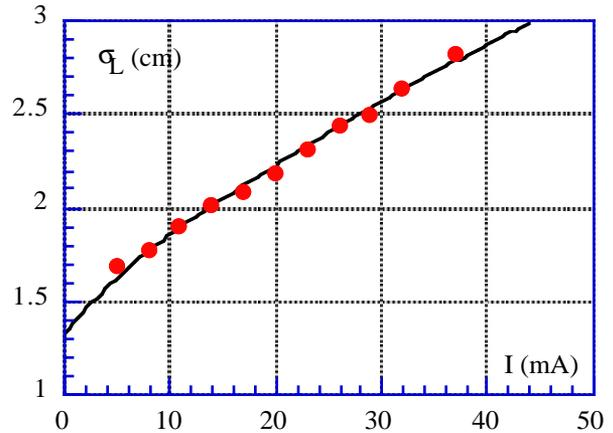
Figure 5: Bunch length simulations (solid line) and measurements (dots) in the  $e^+$  ring
