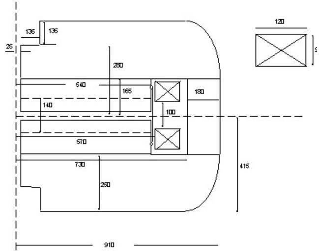
Figure 1: Side view of the 13 MeV cyclotron
