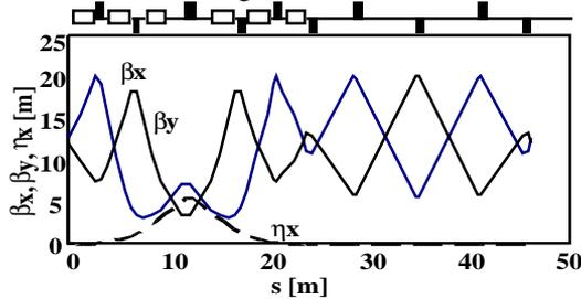
Fig. 2 (a) Beta function and dispersion function of the 20 cell FBDO lattice
