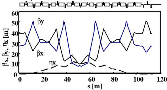
Fig. 1 Magnet lattice for the achromat region in the HEFT
