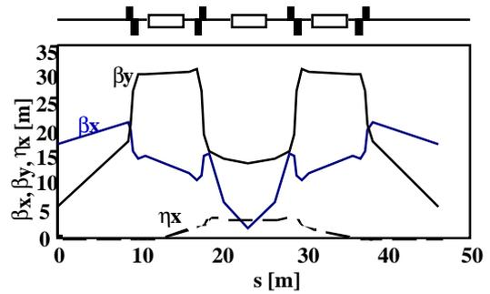
Fig. 2 (b) Beta function and dispersion function of the Triple Bend Achromatic lattice
