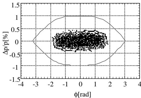
Fig. 3 Beam distribution in a longitudinal phase space
