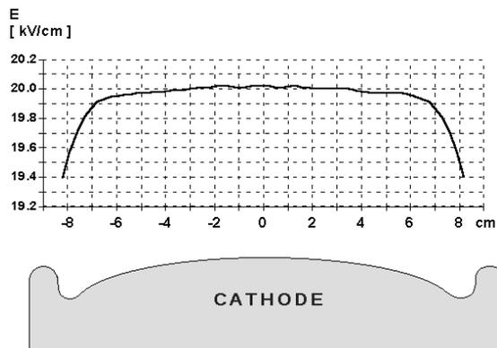
Figure 4: Configuration of the cathode electrode and distribution of the electric field.
