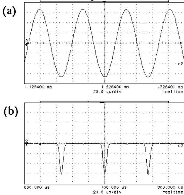
Figure 2: Oscillograms of the accelerating voltage (a) and the electron beam current (b).
