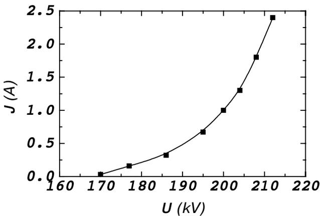
Figure 3: Volt-ampere characteristic of the cold cathode electron gun.
