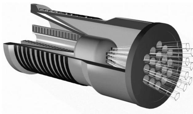
Figure 1: Layout of the multi-beam electron accelerator.
