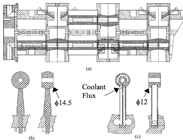
Fig. 1: (a) SCDTL, old design, model #2; Stem arrangement in (b) Model#1 and (c) Model #2
