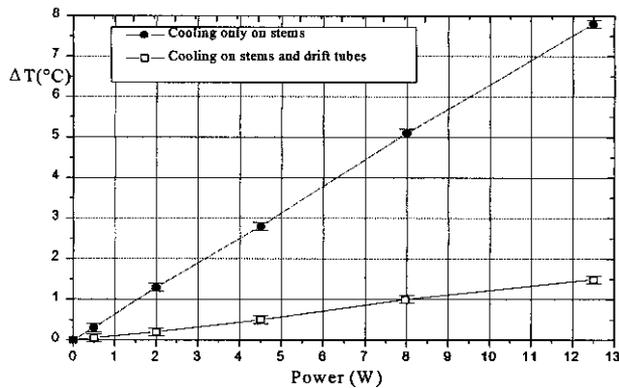
Figure 2: Comparison of the temperature increase in the case of only stem cooling and drift tube and stem cooling
