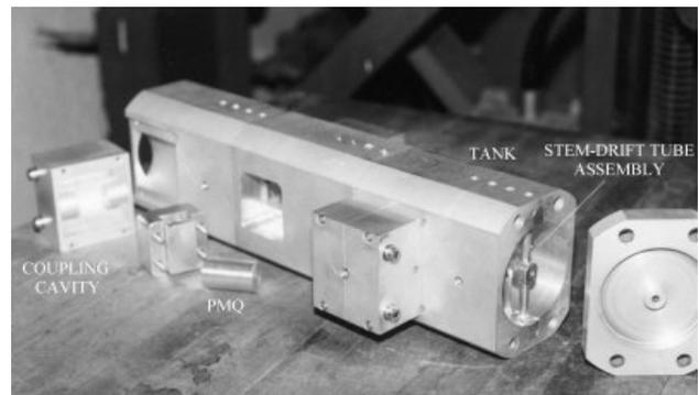
Figure 3: Aluminum model of first three tanks of SCDTL-0
