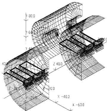
Figure 5: Input geometry for SOPRANO. The stems are in x direction and the z axis coincides with the beam axis.
