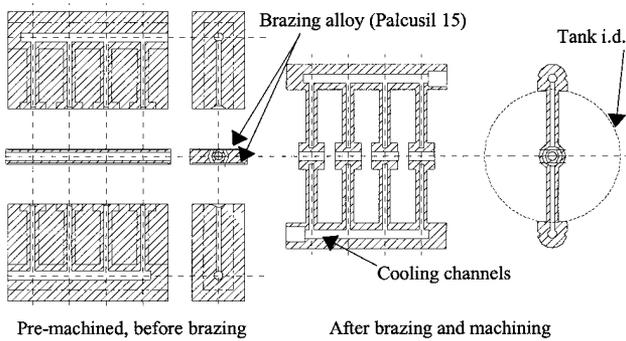
Figure 4: Drawing of the stem-drift tube assembly
