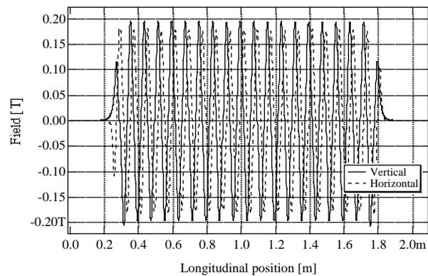
Figure 3 : Horizontal and vertical field components as a function of the longitudinal coordinate for a gap of 16 mm and a current of 250 A.
