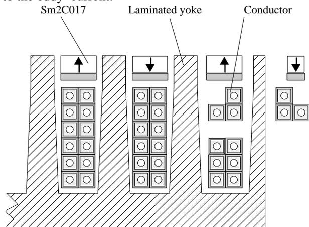
Figure 2: Longitudinal cut of the yoke and coils around the extremity.
