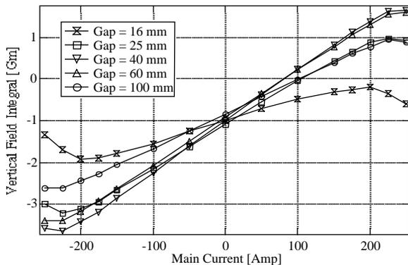
Figure 6 : Average vertical field integral measured as a function of the main current and magnetic gap.
