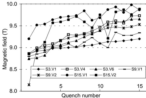
Fig.4 First 15 training quenches of recently tested models
