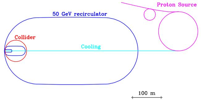
Figure 1: Plan of a 100 GeV Muon Collider.
