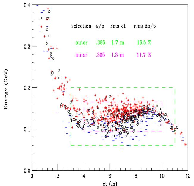
Figure 2: Kinetic energy vs.  $ct$  of muons at end of phase rotation channel. The symbols +, o and - denote muons with polarization  $P > \frac{1}{3}$ ,  $-\frac{1}{3} < P < \frac{1}{3}$  and  $P < -\frac{1}{3}$ , respectively.
