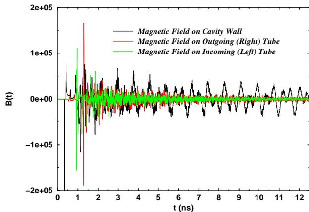
Figure 2: Magnetic field, monitored on different position on the cavity and tube surface
