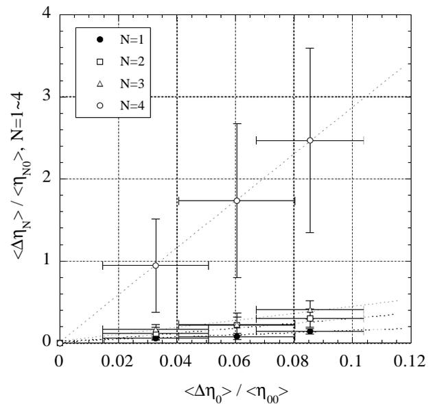
Figure 5: The dependences of the variations of the higher order functions of the nonlinear dispersion on the deviation of the linear dispersion from the design value.
