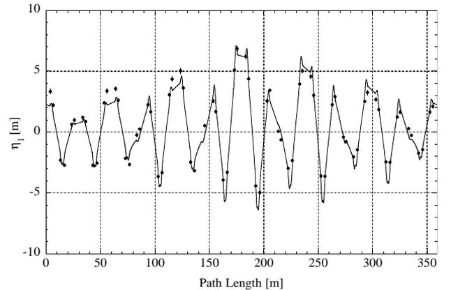
Figure 2: The first order nonlinear dispersion function in a quarter of the storage ring.
