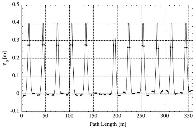
Figure 1: Linear dispersion function in a quarter of the storage ring. The solid line denotes the numerical calculation and the dots the measured values.
