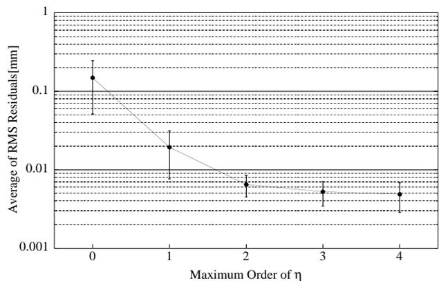
Figure 6: The variation of the average residual of the dispersion function as changing the order of polynomial expansion.
