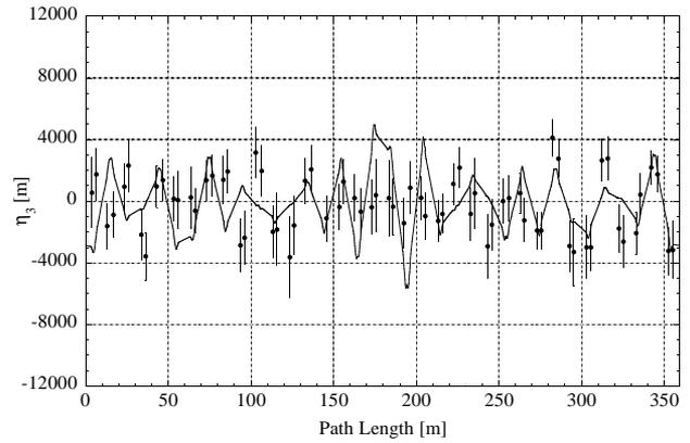
Figure 4: The third order nonlinear dispersion function in a quarter of the storage ring.
