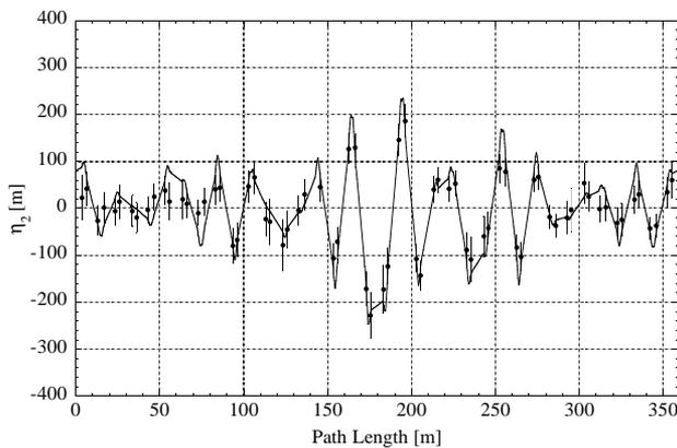
Figure 3: The second order nonlinear dispersion function in a quarter of the storage ring.
