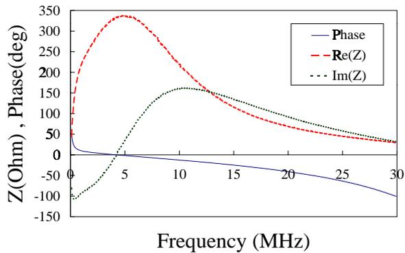
Fig. 5 Impedance curve of the prototype of the high gradient cavity. Total impedance is two times of the value presented in this figure.
