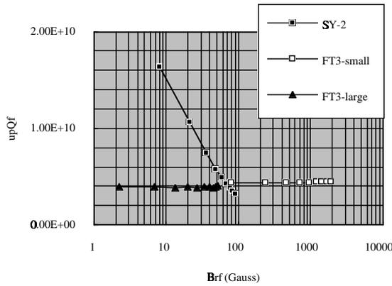
Fig.1 Dependence of  $\mu Qf$  values on the rf magnetic field strength ( $B_{rf}$ ) for Ni-Zn ferrite (SY-2) and magnetic alloy (FINEMET:FT3) cores.
