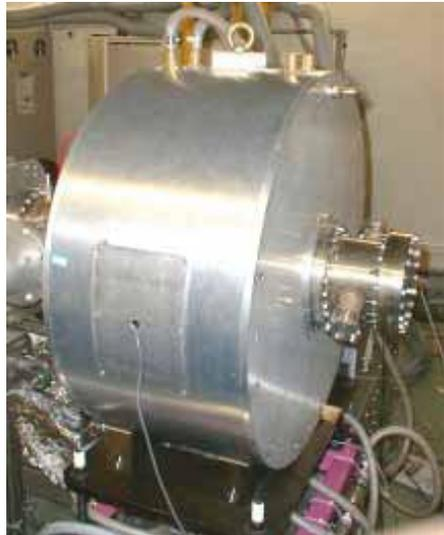
250mm(i.d.) x 670mm(o.d.) x 2.5cm (w). The total length of the cavity including vacuum flanges at the both ends is only 40 cm. In the case of using ordinary cores without
