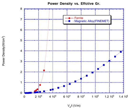
Fig.2 Variation of the power density of the power density as a function of the effective field gradient.
