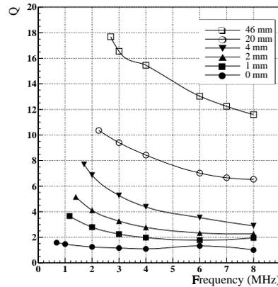
Fig.3 Q-value dependence of the FINEMET core for various radial gap lengths.
