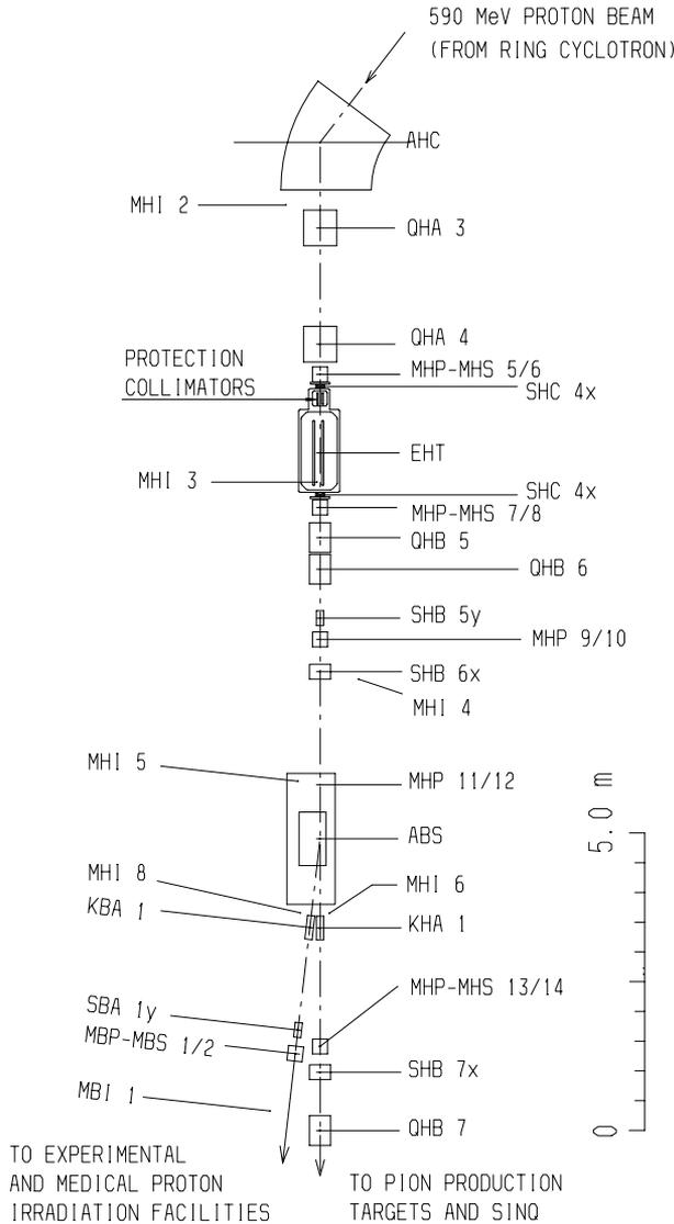
Figure 2: Location of the splitter (EHT) in the 590 MeV B.T.L. The EHT causes the main and peeled-off beams to clear the 20 mm thick septum coil of the C-shaped ABS bending magnet. The M(H,B)(P,S)'s are profile and centre-of-charge monitors. The M(H,B)I's are ionization chambers to monitor beam losses.
