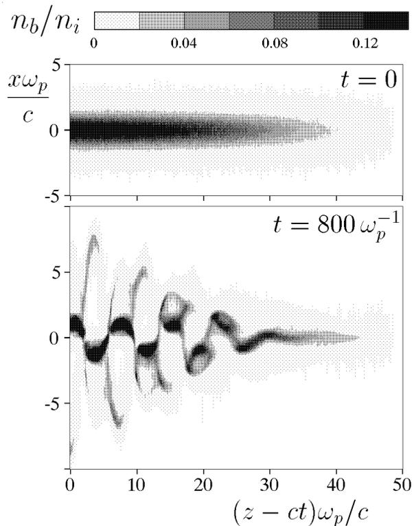
Figure 1: Destruction of the long beam by TTS instability. Plane geometry.
