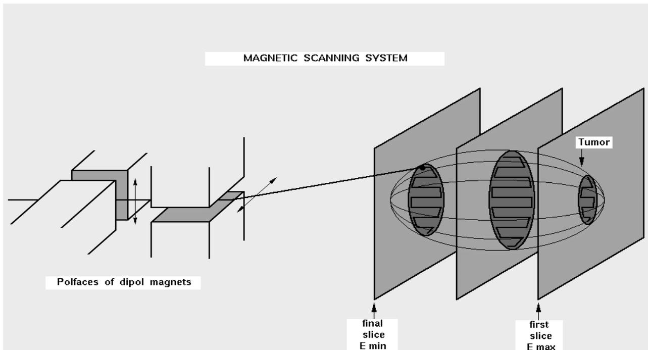
Fig 2. Principle of the rasterscan technique: the target volume is dissected in slices of equal particle range and each slice is painted with a pencil beam in a rasterlike procedure.
