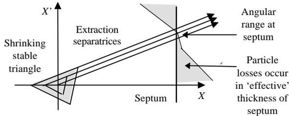
Figure 3: Movement of the extraction separatrix.
