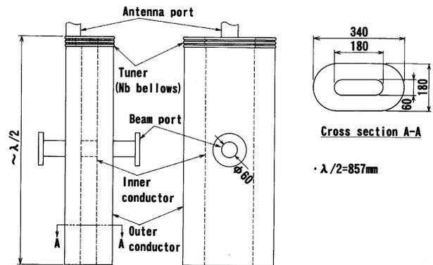
Fig. 1 Optimized sc cavity
