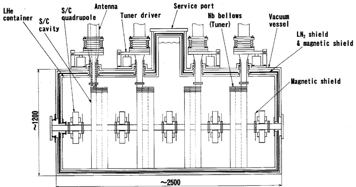
Fig.3 Schematic drawing of the cryounit
