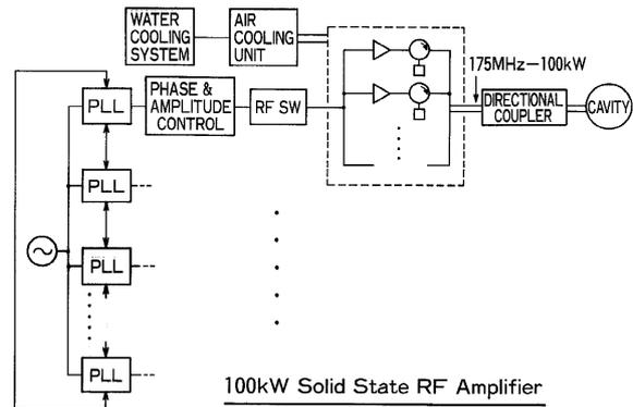
Fig. 5 Schematic diagram of solid state rf amplifier
