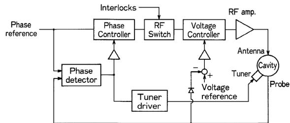
Fig.6 Schematic diagram of rf control system
