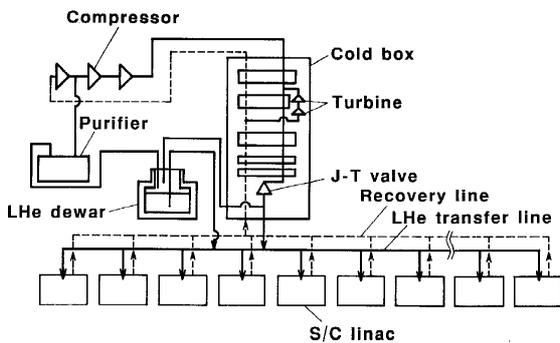
Fig.4 Block diagram of cryogenic system
