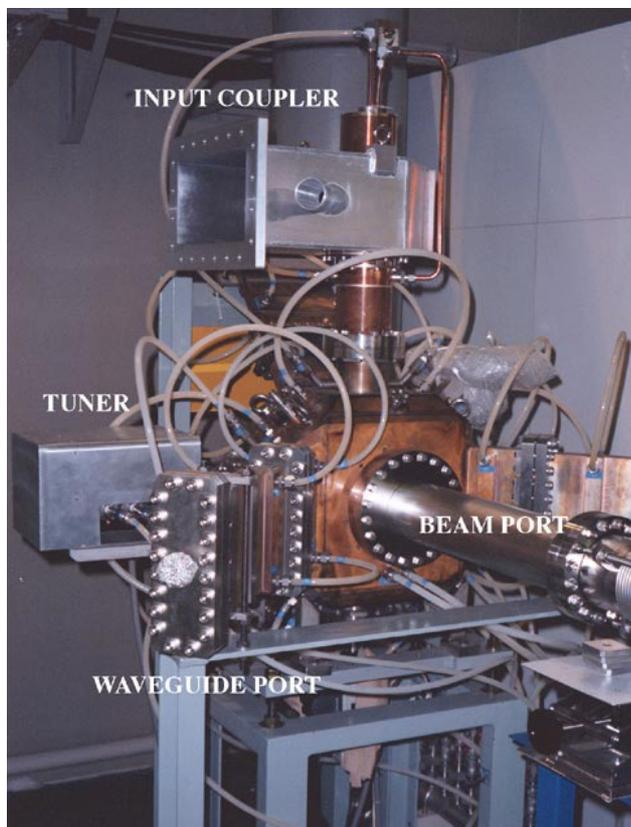
Fig. 1. High-power test cavity mounted on a test bench.
