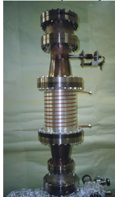
Figure : 2 The SiC duct after pre-baking.
