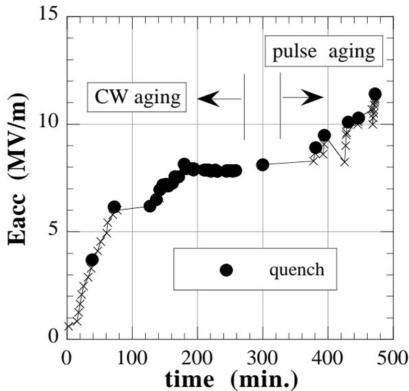
Figure: 2 Aging process in horizontal cold test.
