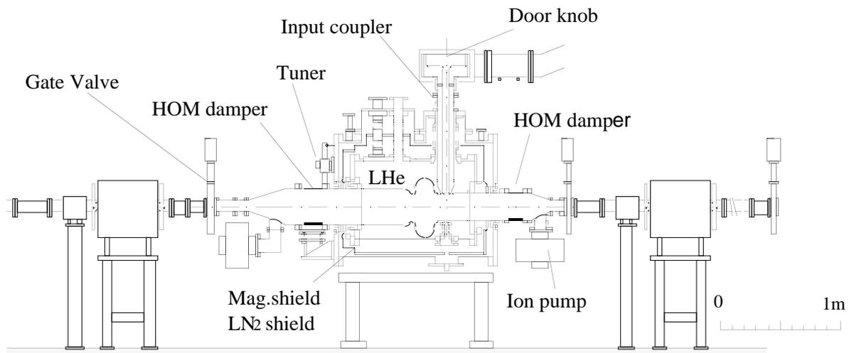
Figure: 1 A sketch of the prototype module in TRISTAN Accumulation Ring.
