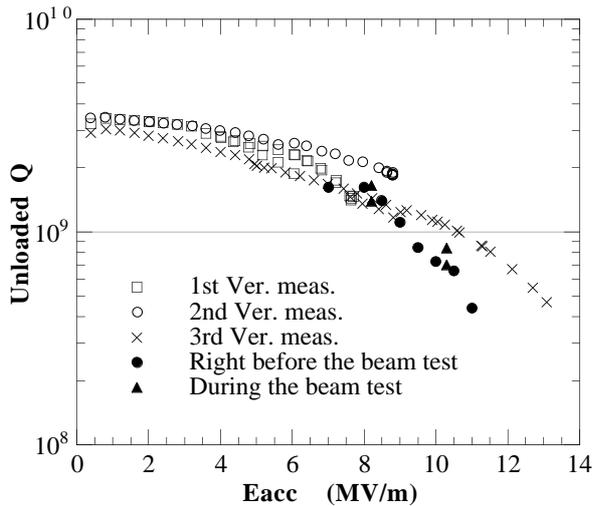
Figure: 3 The Q vs accelerating gradient (Eacc).
