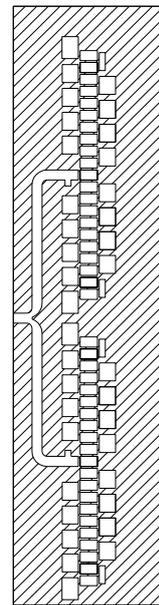
Figure 4: Two structures with central feed line, power splitter and couplers.
