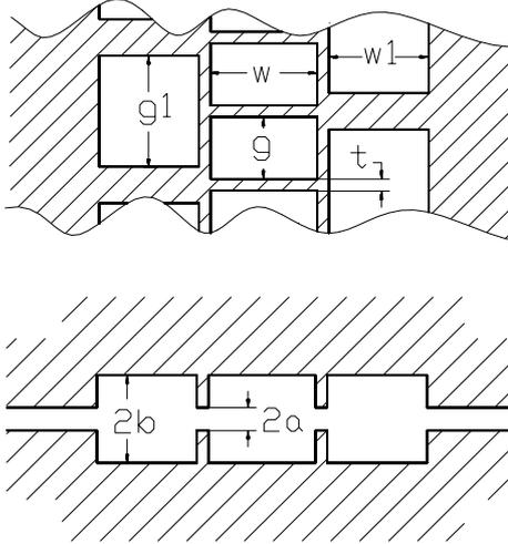
Figure 1: Geometry of the structure:  $g1 = 2.40$ ,  $w = 2.29$ ,  $g = 1.34$ ,  $t = 0.25$ ,  $w1 = 2.14$ ,  $2b = 2.29$ ,  $2a = 0.75$  (in mm)
