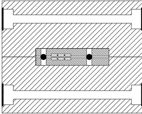
Figure 5: Cross-section of the RF structure with integrated cooling channels.
