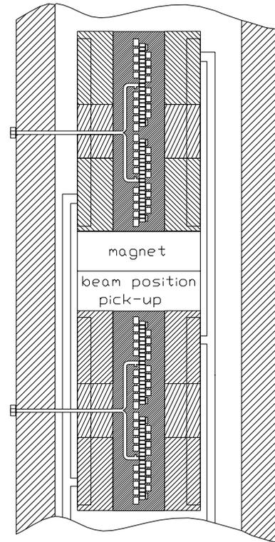
Figure 6: Top-view of the RF structure housed in a vacuum vessel.
