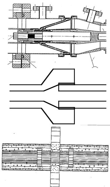
Figure 3 : Conical (upper), cylindrical (middle) and TW disc (bottom) windows
