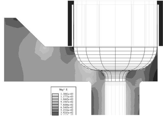
Fig.1 : Doorknob transition with a choke cavity for DC
