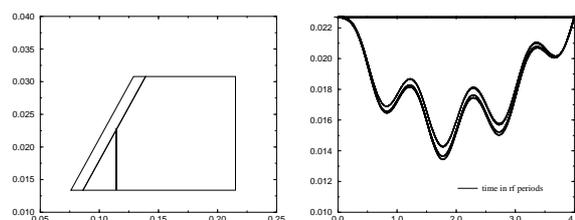
Figure 4 : Multipactor of order 4 involving ceramic in r-z plane (upper) and r-time plane (bottom)
