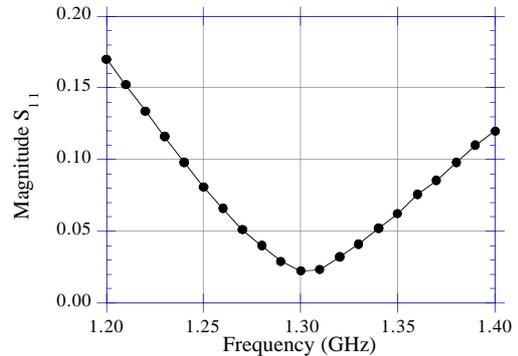
Figure: 2. Reflecting coefficient ( $S_{11}$ ) vs. frequency for doorknob-type transition.
