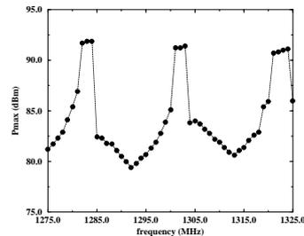
Fig. 6 : Power limitation for a vacuum <math>< 10^{-8}</math> mbar on a waveguide window (pulse length = 200µs).
