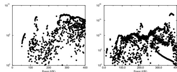
Figure 5 : Total number of emitted electrons after 20 impacts for the conical window at upstream (upper) and downstream (bottom) sides.
