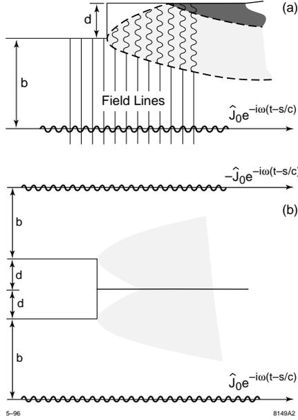
Figure 2: a) Diffacted waves near a step-out transition; b) equivalent geometry with image current.
